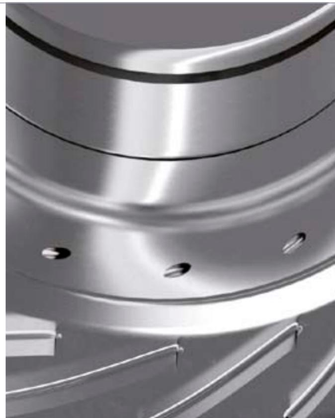
By applying up-to-date 3D CFD and FEA calculations, a new compressor wheel geometry has been created with further improved efficiencies. Depending on the application, part-load and full-load optimisation is possible by means of flow area combinations.
