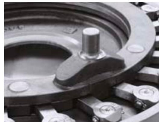
TCR nozzle rings are manufactured from an extremely resistant material which ensures a long service life. Optimum adaptation of the turbocharger to the respective engine is achieved by means of individually selected flow areas (matching).
