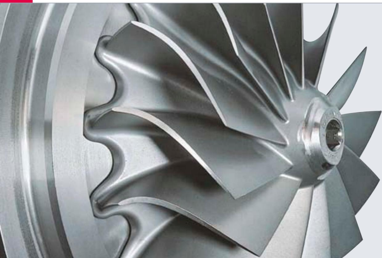
All the flow-through components of the TCR turbocharger have been flow and stress optimised by means of modern 3D-CFD and FEA calculations. Part or full load optimisation is possible by means of a variety of different rotor/nozzle ring flow area combinations.
