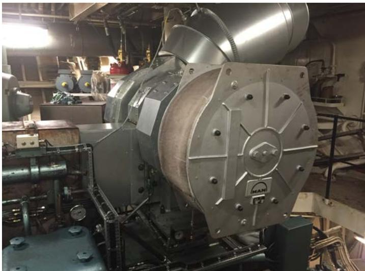
*Alternate views of the newly retrofitted radial MAN TCR20 turbocharger*
